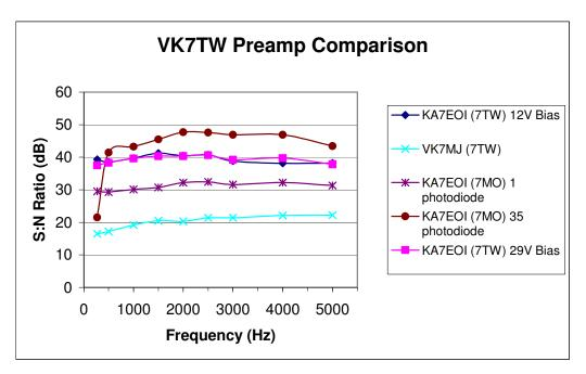
On 18 November 2007 a comparative field test was undertaken between the VK7MO built 35 photodiode array using the KA7EOI design behind a 320x400mm Fresnel lens and the VK7TW built one photodiode KA7EOI design in the focal point of a 320mm mirror dish via cloud bounce on a 27km path between VK7MO and VK7DY's QTHs. More information can be found at: http://reast.asn.au/optical/Field\_Comparisons\_VK7MO\_VK7TW\_VK7DY\_20071118.pdf
