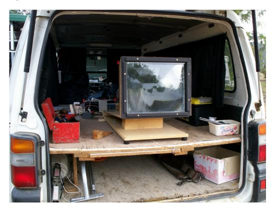
Ken used a Laptop and external battery pack to provide several hours operation without any hum problems as occur with switch mode power supplies. The Receiver was aligned by transmitting a tone and peaking azimuth and elevation on Spectran in a bandwidth of 0.084 Hz.
