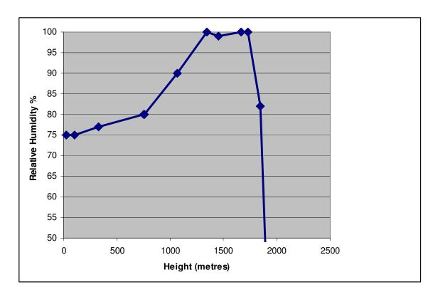
It is seen that the Relative Humidity reached 100% at around 1350 meters consistent with the cloud height given by the airport reports. 1350 meters provides a useful window to transmit light over the Meehan range at 300 to 350 metres around 10 km from Rex's QTH.
