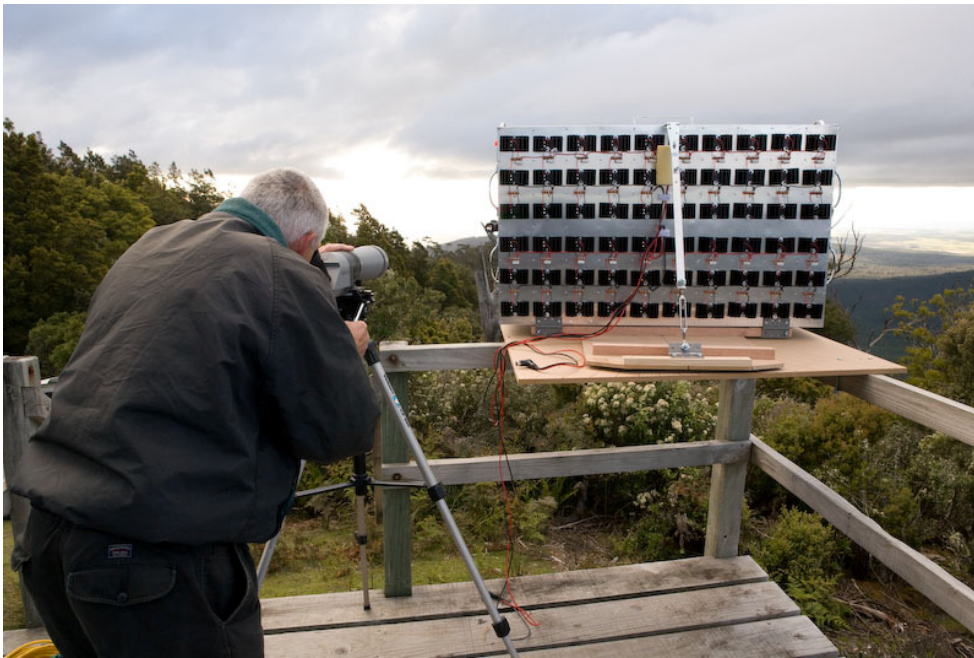
Fig 3: Rear View of new TX showing 60 Luxeon Heat sink mounts and Azimuth and Elevation arrangement, also VK7JG – Photo courtesy of Alvin VK7NDQ
