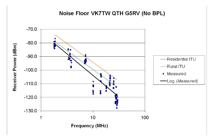
Noise floor measurements for 1.8, 3.5, 7, 10, 14, 18, 21, 24 & 28MHz undertaken using the <u>FSM application</u>, Yaesu FT-847 and G5RV 104foot dipole, prior to the installation of BPL equipment in September 2007 in Wentworth St, South Hobart, Tasmania, Australia. "Residential and Rural ITU" are the expected ambient noise levels (ITU-R P.372-8) for a residential and rural area for a bandwidth of 2481Hz for comparison purposes.
