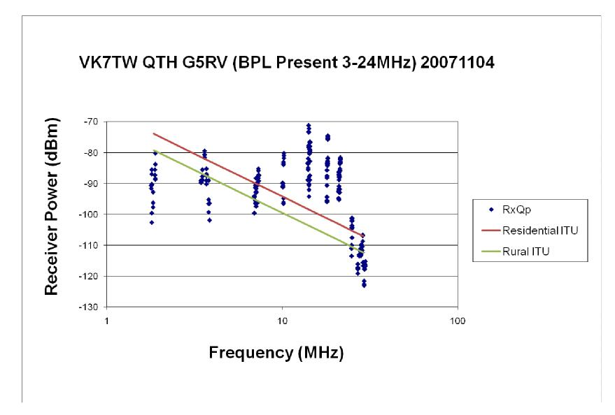
BPL noise measurements for 1.8, 3.5, 7, 10, 14, 18, 21, 24 & 28MHz undertaken using the <u>FSM application</u>, Yaesu FT-847 and G5RV 104foot dipole on 4 November 2007 in Wentworth St, South Hobart, Tasmania, Australia. Please note: BPL band plan covered the 3-24MHz spectrum and quasi-peak measurements used.
