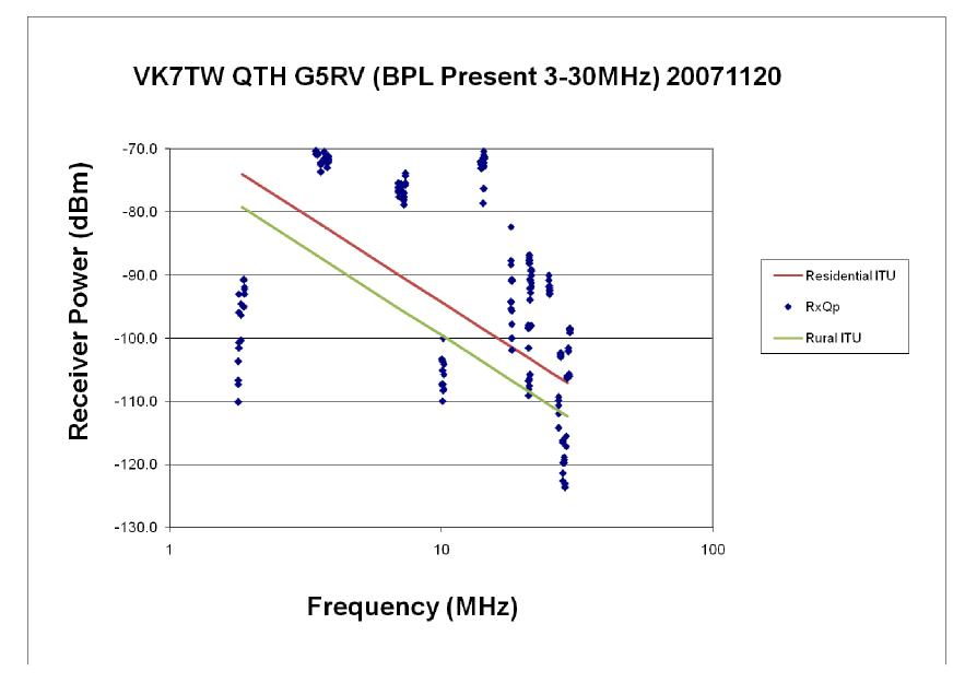
BPL noise measurements for 1.8, 3.5, 7, 10, 14, 18, 21, 24 & 28MHz undertaken using the <u>FSM application</u>, Yaesu FT-847 and G5RV 104foot dipole on 20 November 2007 in Wentworth St, South Hobart, Tasmania, Australia. Please note: BPL band plan covered the 3-30MHz spectrum and quasi-peak measurements used.
